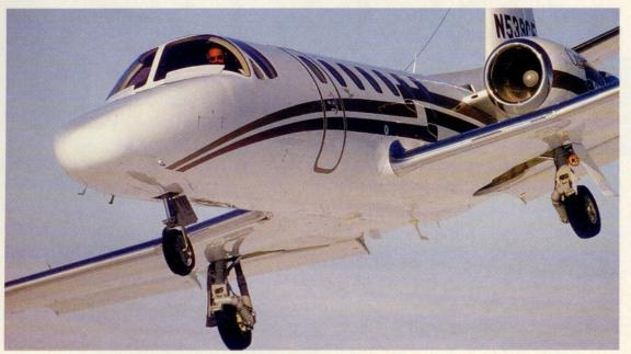
More powerful PW535 turbofans, a longer wingspan, full-span bleed-air anti-ice panels, and trailing-link landing gear distinguish the new Citation Encore. The standard, threetube Honeywell Primus 1000 avionics suite—with a standby Meggitt combination attitude indicator/HSI color LCD—gives the Encore an additional edge over its predecessors.
